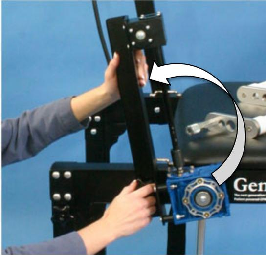
5. With the hand-crank assembly removed, unscrew the black knob on the right arm and remove the bolt. Rotate the arm up into position. (It will be necessary to rotate the round drive shaft to move the leg in order to allow the arm to tilt.) Replace the bolt and firmly tighten the black knob.
